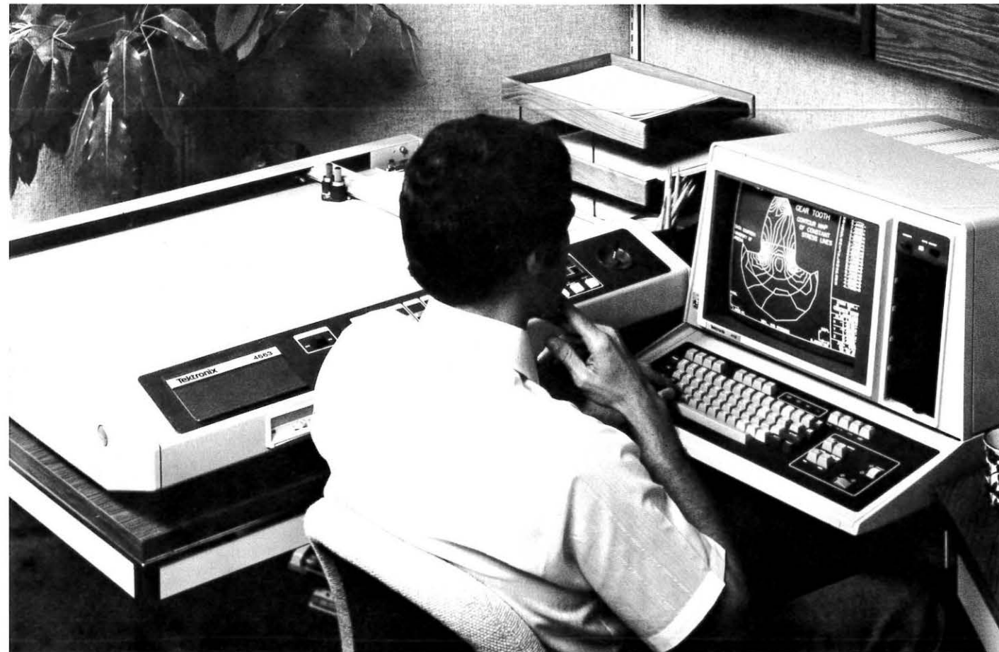
This Tektronix 4112 computer display terminal is a monochrome raster display device combining graphics with powerful local intelligence to provide users with high interactivity and low host
