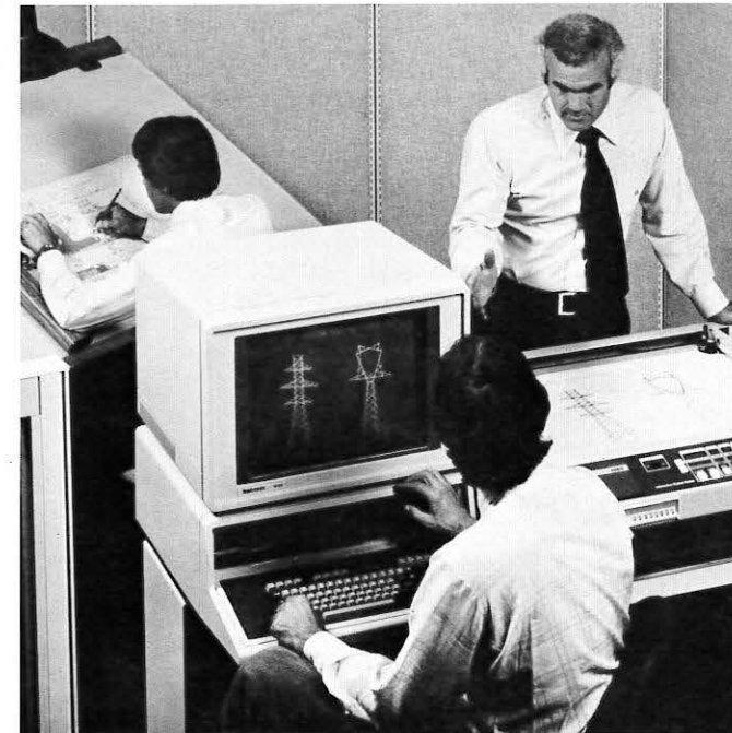
This new Tektronix 4114 computer display terminal is described by the maker as combining the high information density of a 19-inch direct view storage tube with powerful local intelligence, local refresh, and fast transmission and redraw.
